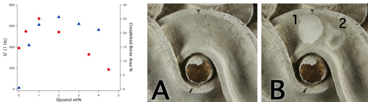
Figure 2: On the left, Storage modulus values at Frequency=1Hz (■) and Crosslinked Borate Area obtained from NMR measurements (▲) are plotted against glycerol concentration. Pictures on the right show the stucco surface before (A) and after (B) the cleaning, with the comparison between the the HPG based system (1) and a wet cotton swab (2).
