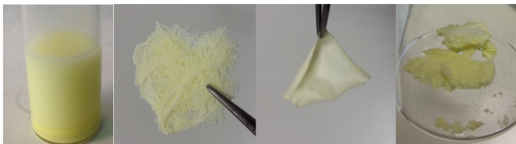
Figure. (From left to right) Nanoparticles dispersed in a solvent, Ce:YAG composites in glass wool, filter paper and cotton wool.
