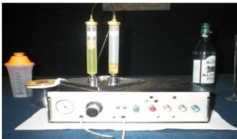
FIGURE 1. Laboratory prototype of Esxtractor Naviglio (1998).
